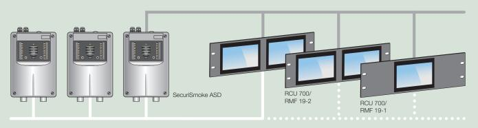
Up to 100 SecuriSmoke ASDs can be shown on a RCU 700. The assignment can be freely selected according customer wishes and the project.
